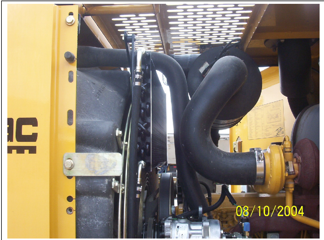
Add on pulley fastens to crankshaft. Belt on outside groove of compressor.
