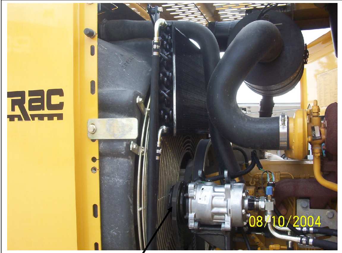
Add on pulley fastens to crankshaft. Belt on outside groove of compressor.
